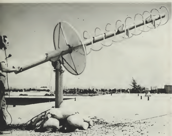
5. Electronic devices inside the missile send back critical data which are picked up by telemetry antennas like this one.
