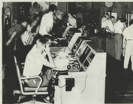
6. Information is sent to Operations Room where officer can destroy missile electronically if it veers off course.
