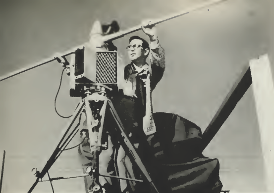
3. Missile's takeoff is recorded by as many as 75 special cameras, like this Fairchild Analyzer aimed by binocular sights.
