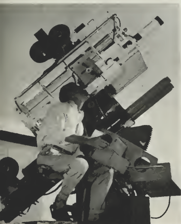
As missile soars down-range, it is followed by high-speed, long focal-length cameras like this tracking telescope mount.
