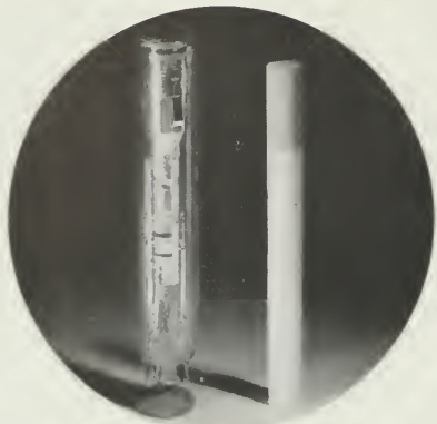
At heart of RCA's new transistorized TV camera is this RCA-developed 1/2-inch Vidicon tube, shown here in comparison with a king-size cigarette. Tube is now being produced in sample quantities.
