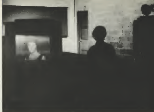
In semi-darkness, the RCA wide-spaced image orthicon TV camera tube picks up and displays clearly the image of a human model.
