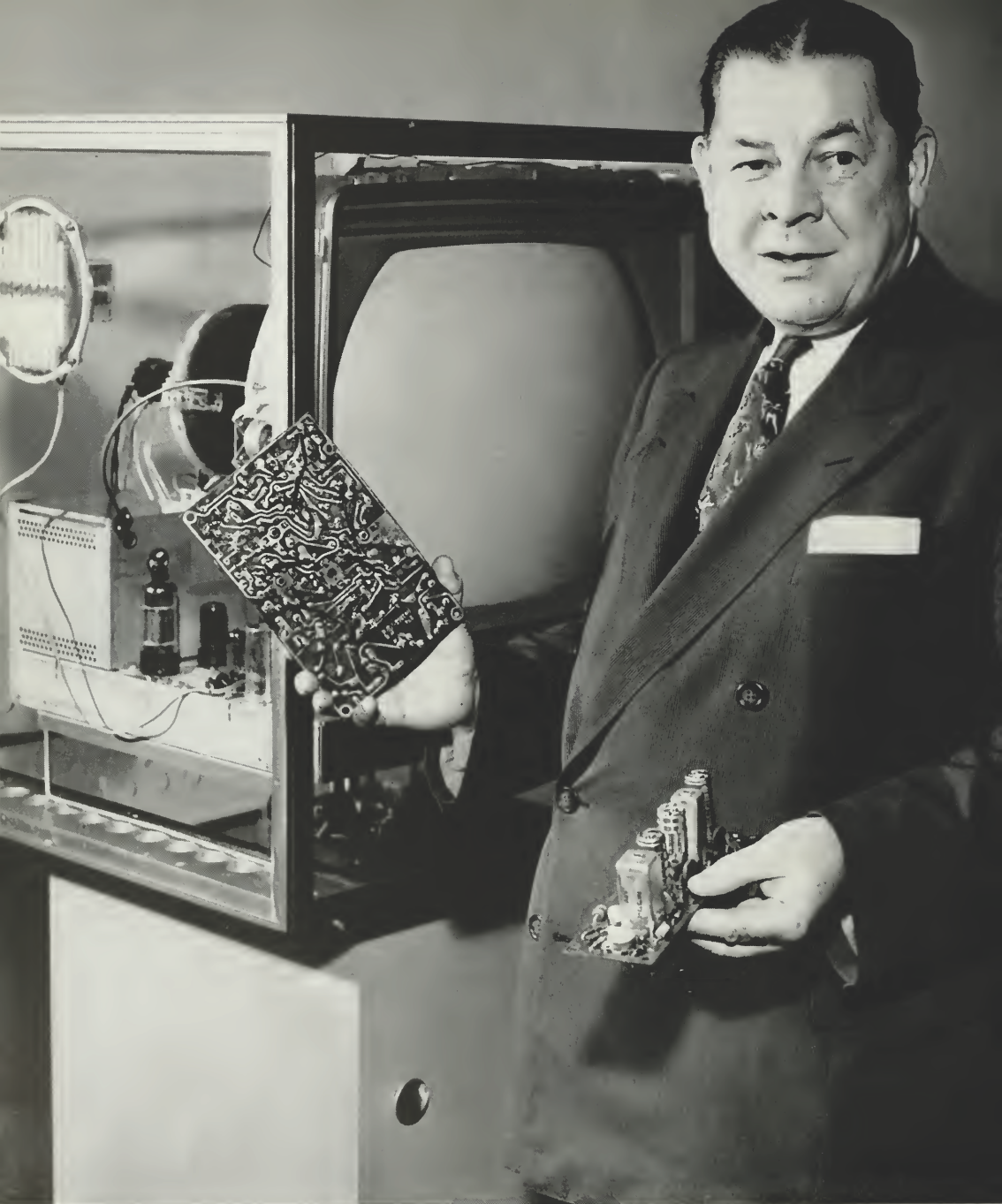
FOR MASS PRODUCTION—Two of the printed circuit boards used in the new RCA Victor color TV sets are displayed here by Robert A. Seidel, Executive Vice-President, RCA Consumer Products.
