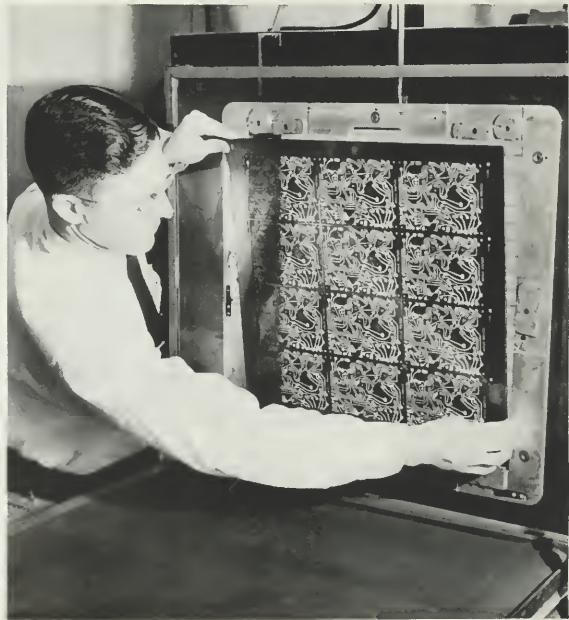
2. Photo-master is used to produce a glass negative, seen here being inserted in photo contact printer. The negative contains a number of duplicate patterns.
