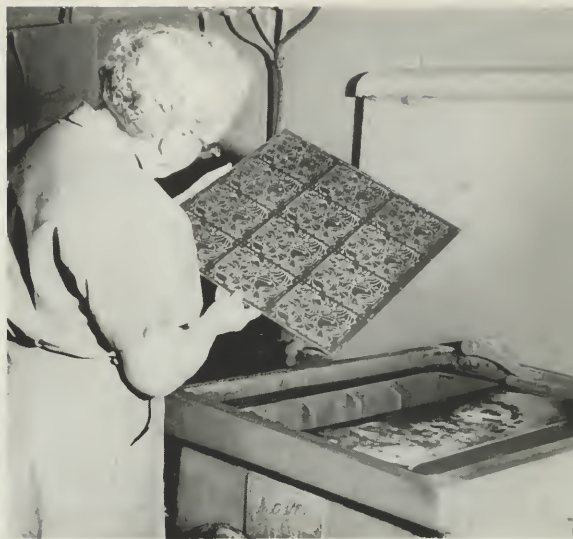
4. Exposed board is then developed photographically and put through an etch bath which dissolves unexposed copper, leaving replica in copper of the original circuits.
