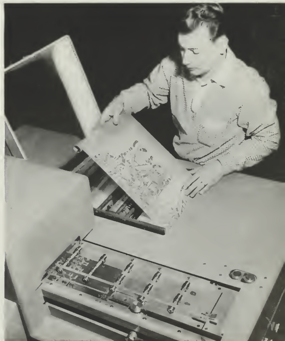
6. Each printed circuit board is punched to provide for insertion of components. RCA's Programmed Punch Press, (above) can punch virtually any pattern.
