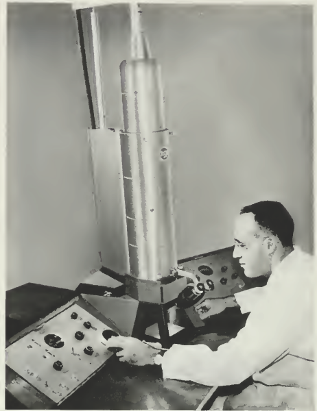
A leading electronic contribution to medicine is RCA's electron microscope, shown here in operation at Armed Forces Institute of Pathology, Washington.
