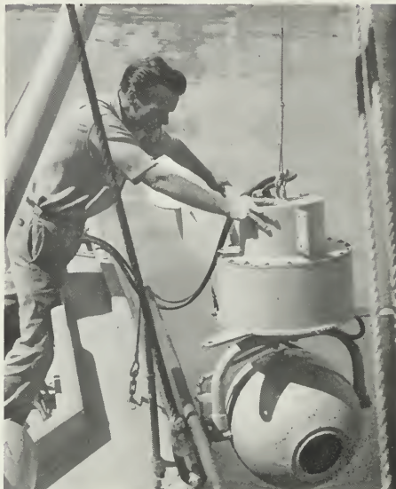
Reidar F. Sand, of U. S. Fish and Wildlife Service, readies diving bell which houses RCA TV camera used to observe fishery gear under water.
