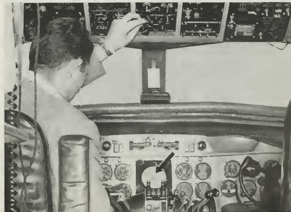
Nose of UAL Convair has been extended 28½ inches to house antenna and gear mechanism of RCA weather radar. Below, engineer checks radar installation in plane cockpit. Arrow indicates radar scope.
