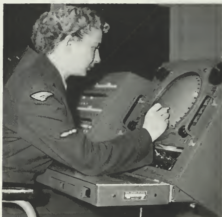
On a plan position indicator scope, a member of the staff at one of the radar stations maintains watch.
