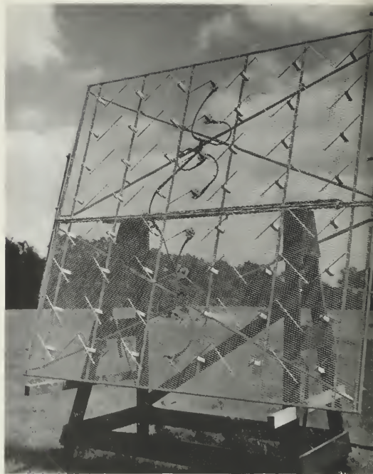
Receiving antenna of the RCA experimental UHF booster station, shown at Princeton before shipment to Vicksburg for the successful six-weeks trial.
