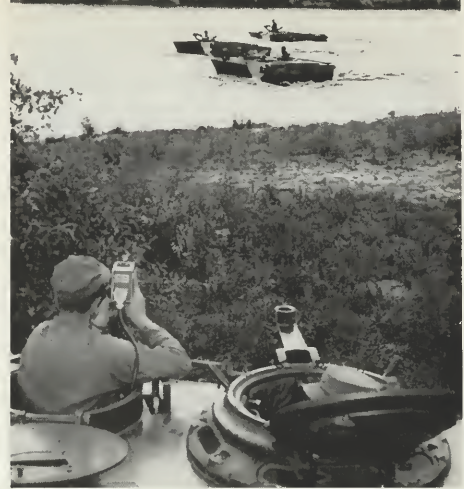
Above, TV combined with the Army's new long-range lens may give instantaneous view of distant objectives. At right, combat TV camera mounted on amphibious vehicle covers start of mock assault across lake at Fort Meade.
