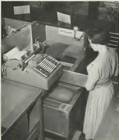
Largest installation yet of "TV Eye" helps to speed banking operations at the Provident Institution for Savings in Boston. File clerk, above, holds signature card before the camera for viewing by teller, right.
