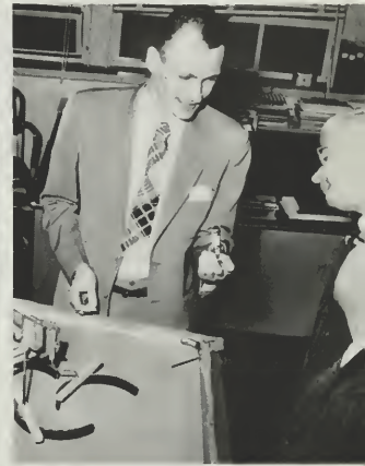
Robert Anderson shows device used to chart path of electrons in a tube.
