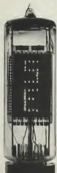
Selective electrostatic-type storage tube with capacity of 256 units.
