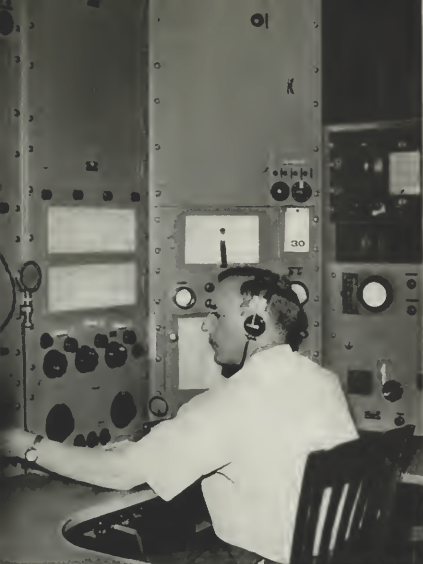
Technician F. B. Kennell at the main operating position of RCA's frequency measuring laboratory tunes a radio station which is to be checked for accuracy of transmissions.
