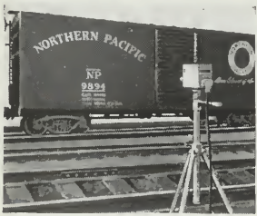
In a railroad yard, RCA vidicon camera lets employees check car numbers at long range.
