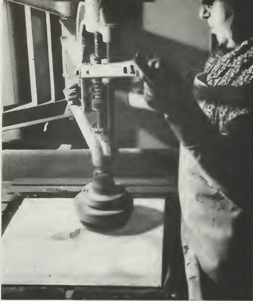
A copper-clad sheet of plastic, on which electronic circuits will be printed by photography, is highly polished before the light-sensitive emulsion is applied.
