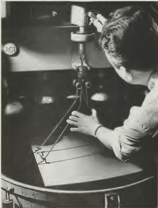
In this heat tank, the sensitized copper-clad plastic sheet is dried rapidly under a bank of infra-red lamps and over a row of gas burners.
