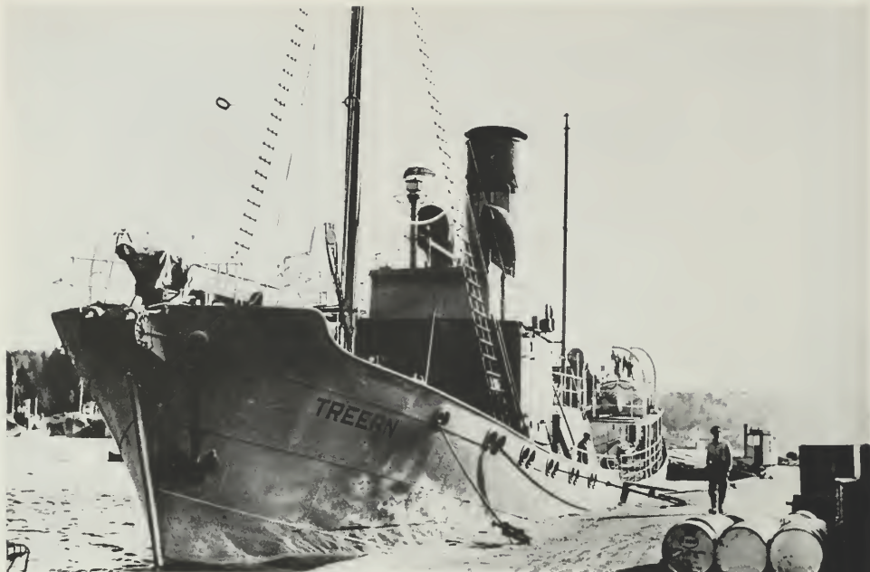
The Treern , a typical whale "catcher", is one of a fleet of 55 vessels equipped with RCA radar for a Norwegian whaling firm. The radar antenna, indicated by the circle, is installed above the bridge deck.
