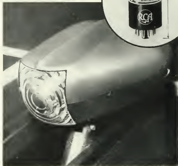
Autronic Eye, containing small light-sensitive tube (insert), electronic relay and control circuits, automatically depresses bright beam when one or more cars approach and raises beam when traffic has passed.
