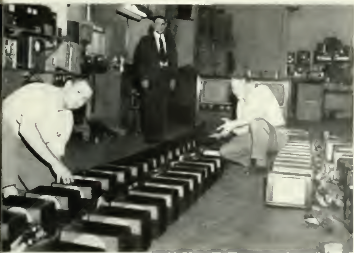
Rows of table model radio sets (above) and new television receivers (below) are subjected to on-and-off tests for 100 hours or more while technicians watch for any deviations from RCA standard of quality.
