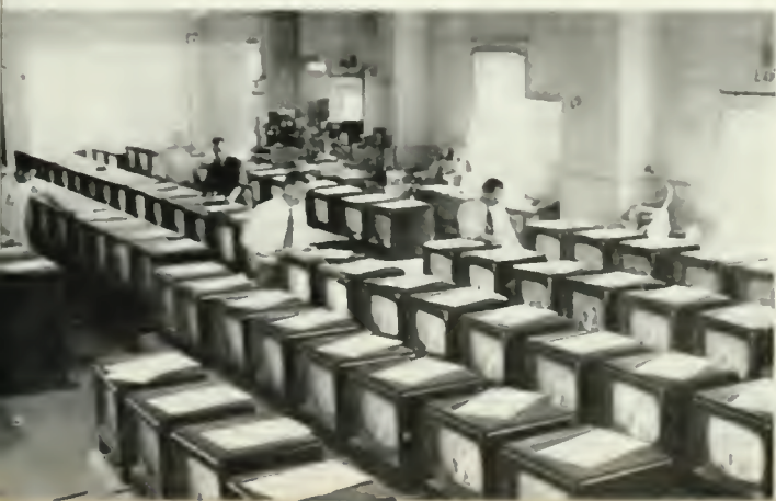
Rows of table model radio sets (above) and new television receivers (below) are subjected to on-and-off tests for 100 hours or more while technicians watch for any deviations from RCA standard of quality.
