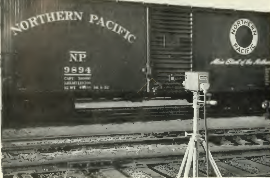
An RCA industrial TV camera scans passing freight cars and transmits the moving images to a recorder who notes the car numbers and other essential data.
