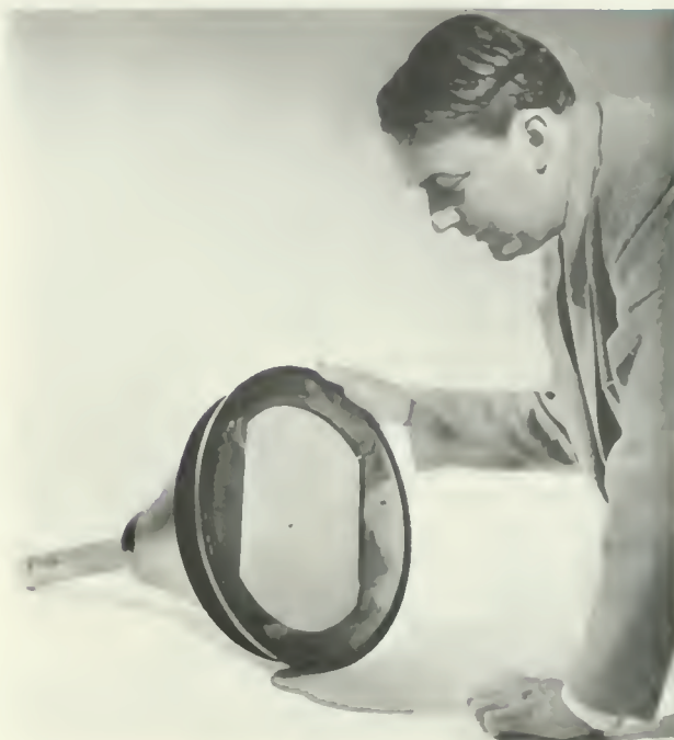
Alfred C. Schroeder and one of the RCA tricolor TV tubes which utilize his invention.
