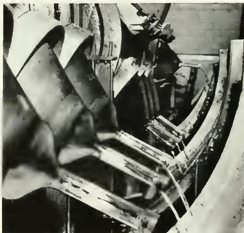
At the end of the settling belt, automatic machinery tips the tube and decants the remaining liquid.
