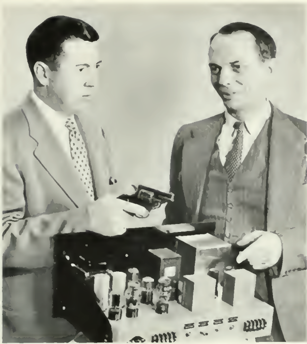
R. E. Lofferty (left) and J. L. Hothaway, NBC engineers, demonstrate the electronic "gun-shot reinforcer" which they developed for radio and TV dramas.
