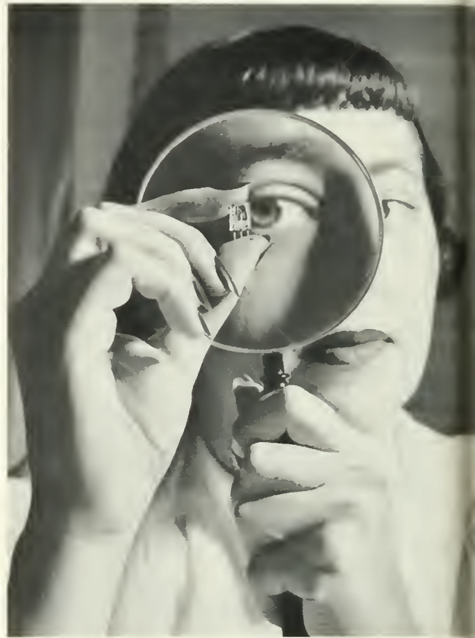
Although only the size of a kernel of corn, the transistor performs the functions of certain types of vacuum tubes.
