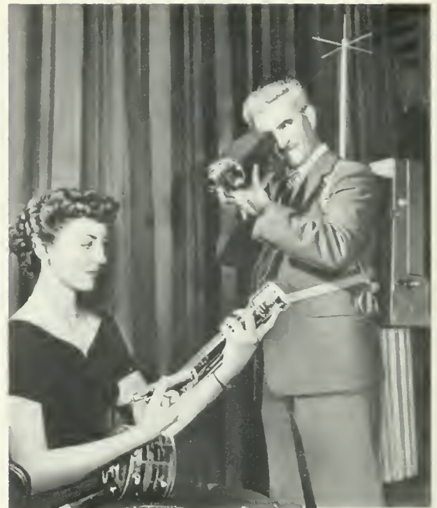
Development of Vidicon tube (in girl's right hand) made possible the back-pack TV transmitter shown at right.
