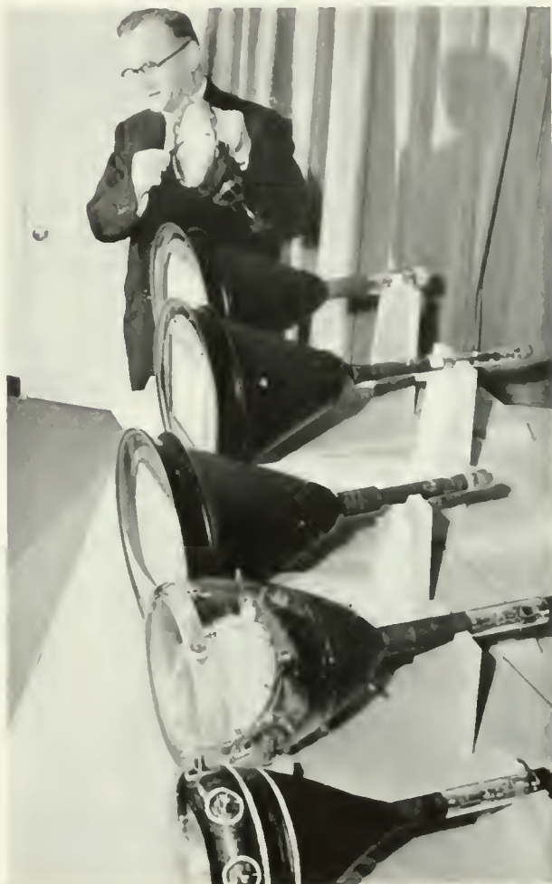
The author points to one type of tri-color television picture tubes developed by RCA.
