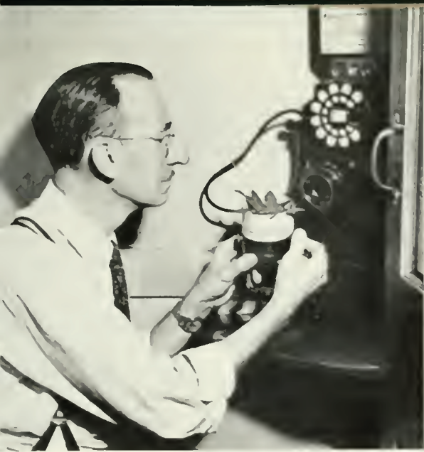
A telephone booth provides the minimum atmospheric noise for recording the delicate sounds of beetles chewing leaves.
