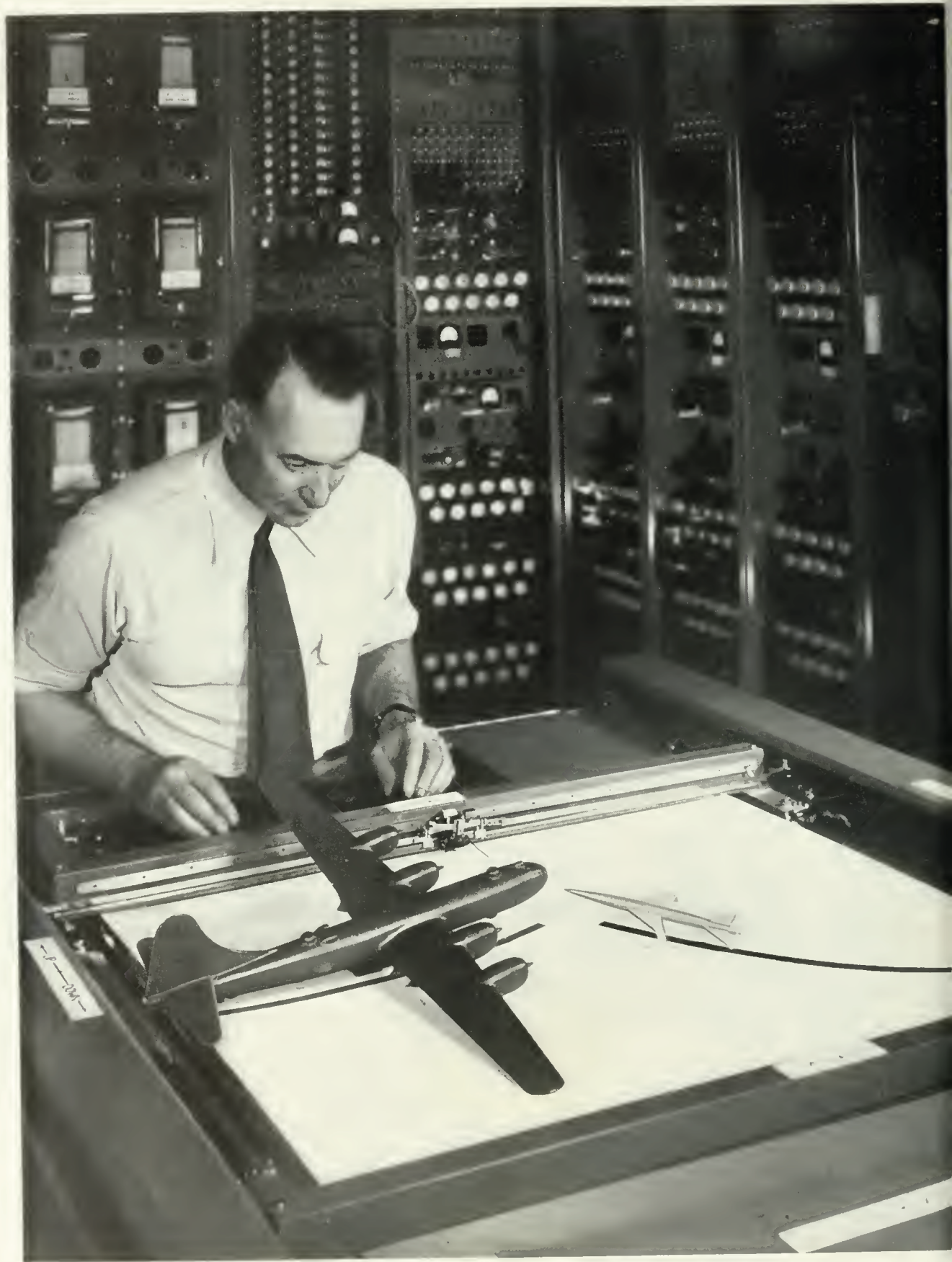
MODELS OF GUIDED MISSILE AND "ENEMY" BOMBER ABOUT TO MEET IN A DEMONSTRATION OF THE ELECTRONIC ANALOGUE COMPUTER DEVELOPED AT RCA LABORATORIES.
