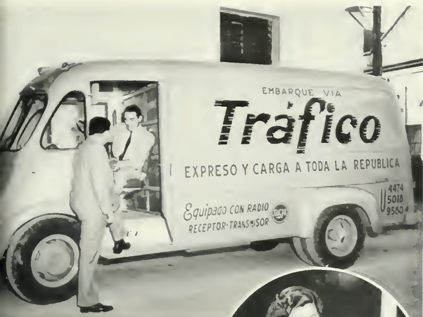
USING RCA MORILE-RADIOTELEPHONE UNITS, INSTALLED IN EIGHT TRUCKS OF CUBA'S LARGEST EXPRESS FIRM, DRIVERS CAN RECEIVE INSTANT INSTRUCTIONS FROM HEADQUARTERS.
