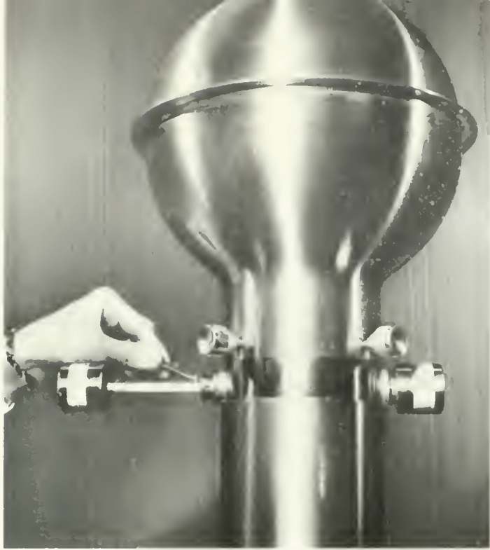
SPECIMENS TO BE OBSERVED IN THE TABLE MODEL ELECTRON MICROSCOPE (SEE FRONT COVER) ARE INSERTED INTO THE INSTRUMENT THROUGH THE SMALL ROD SHOWN ABOVE.
