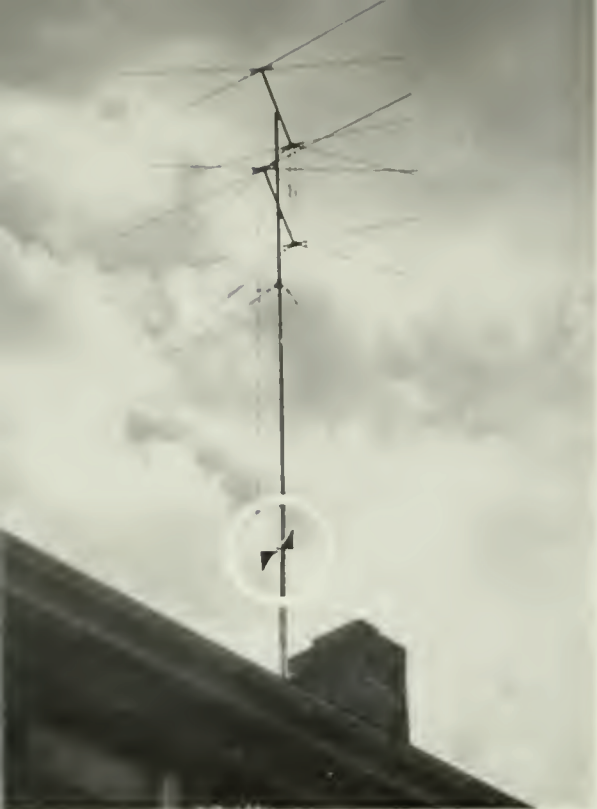
"BOW-TIE" ANTENNA (IN CIRCLE) IS ONE OF SEVERAL TYPES OF UHF RECEIVING ANTENNAS UNDERGOING TESTS IN THE BRIDGEPORT AREA.
