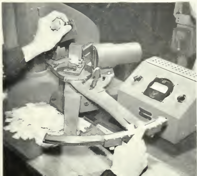
EACH CRYSTAL IS SUBJECTED TO X-RAYS TO DETERMINE THE ACCURACY OF THE SAWING PROCESS TO VERY CLOSE TOLERANCES.
