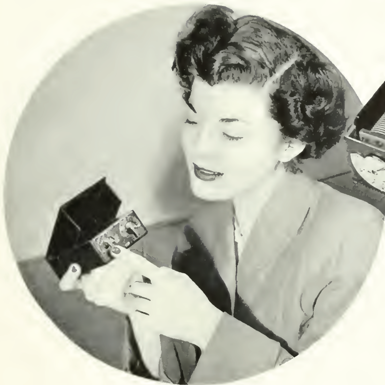
CONTAINING FOUR MINIATURE TUBES AND ALL BATTERIES, THE RECEIVER IS SMALL ENOUGH TO FIT EASILY INTO A POCKET OR MILADY'S HANDRAG. BELOW: COMPARISON OF PREVIOUS "PERSONAL" RADIO AND THE LATEST MODEL.
