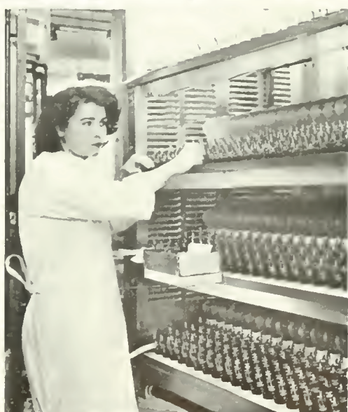
AT THIS AGING RACK, EVERY MINIATURE TUBE IS STABILIZED TO ASSURE ITS LIFE-TIME UNIFORM OPERATION.
