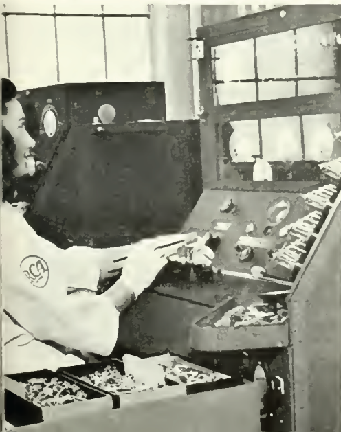
WRAPPING THE TUBE WITH A SMALL Mallet REVEALS ANY IMPERFECTIONS IN ELEMENTS AND THEIR CONNECTIONS.
