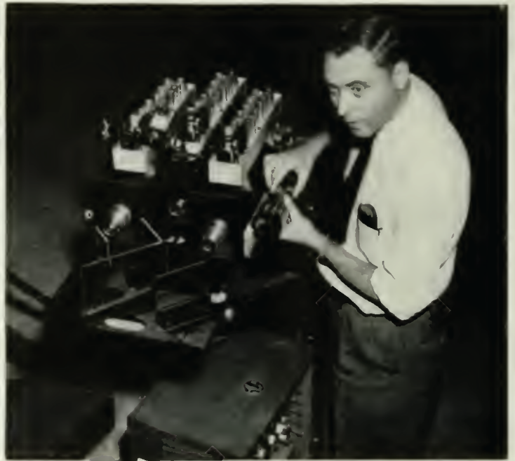
LEFT: RCA COLOR CAMERAS OPERATING IN STUDIO OF WNBW, WASHINGTON, D.C. BELOW: NEW COLOR TELEVISION CAMERA WITH COVER REMOVED SHOWING DICHOIC MIRRORS (IN FRONT) AND SOME OF THE CAMERA'S ELECTRONIC CONTROLS.
