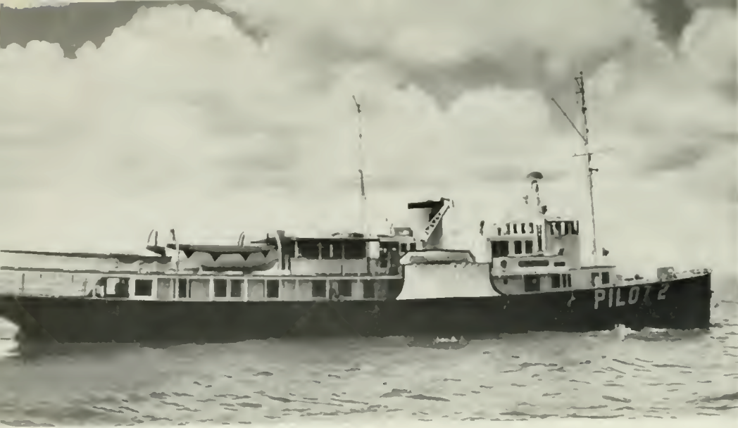
PILOT BOAT NEW JERSEY, SHOWING THE UNUSUAL "HALO" ANTENNA AMID-SHIP WHICH PICKS UP TELEVISION SIGNALS FROM NEW YORK AND PHILADELPHIA REGARDLESS OF THE POSITION OF THE SHIP WHEN STATIONED OFF NEW YORK HARBOR.
