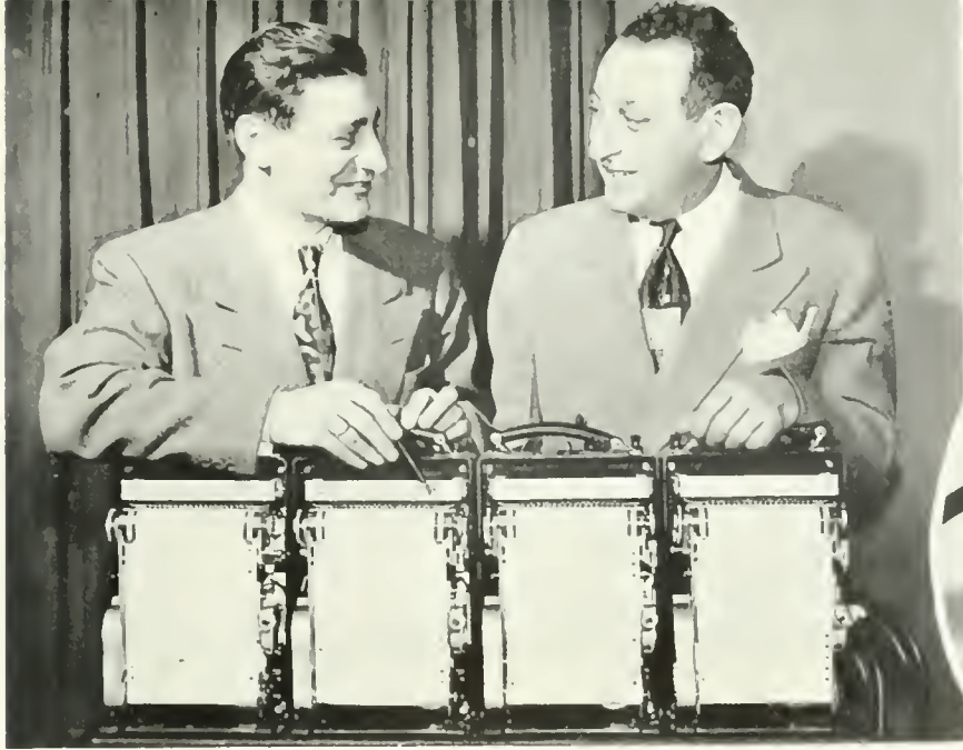
RICHARD PAIGE AND HORACE SCHWERIN DISPLAY THE "TV REACTION RECORDER" WITH ITS 80 TRACING PENS EACH OF WHICH IS CONNECTED TO A "TEST TRIGGER" MANIPULATED BY A MEMBER OF THE STUDIO AUDIENCE.
