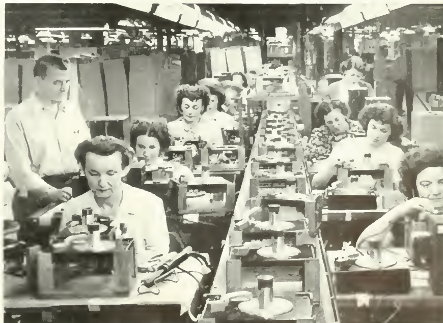
6 A moving conveyor separates the assembly group on the left from testers and inspectors of the finished product on the right.
