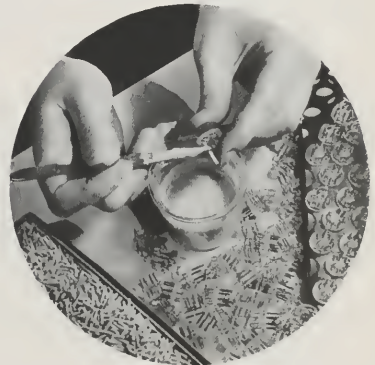
CEMENTING CERAMICS INSULATION IN MINIATURE TUBE MANUFACTURE CALLS FOR STEADY HANDS AND KEEN EYESIGHT.
