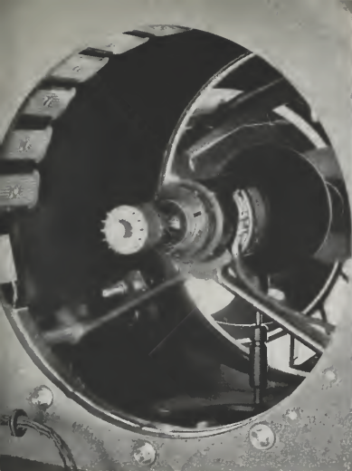
FRONT OF LARGE SCREEN TELEVISION PROJECTOR SHOWING CATHODE RAY TUBE AND THE 30-INCH SPHERICAL MIRROR IN REAR OF OPENING.
