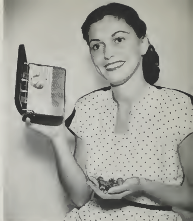
MINIATURE TUBES MADE POSSIBLE THE COMPACT "PERSONAL" RADIO.
