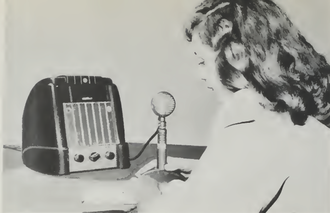
NEW WIRE RECORDER PLAYS FOR 30 MINUTES USING CARTRIDGE WHICH SIMPLIFIES THE HANDLING OF THE SPOOLS OF WIRE CARRYING SPEECH OR MUSIC.
