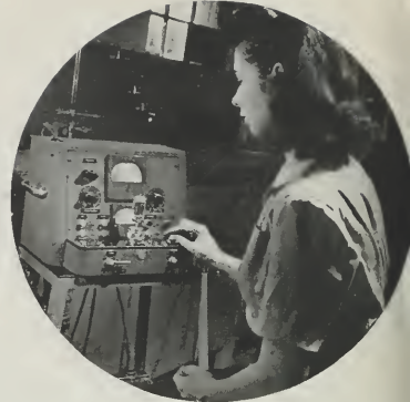
THIS DETECTOR USING NEW VACUUM GAUGE TUBE LOCATES LEAKS SO SMALL THAT MOLECULES OF AIR CAN SCARCELY PENETRATE THROUGH OPENINGS.
