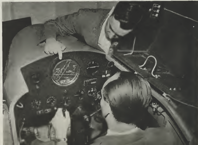
TELERAN SCOPE ON INSTRUMENT PANEL OF PLANE, SHOWING AIR ROUTES AND TERRAIN INFORMATION SUPPLIED FROM GROUND STATION.
