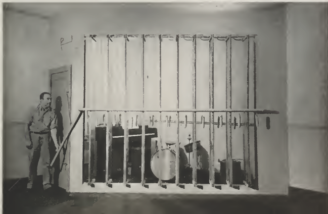
ACOUSTICAL FILTERS USED IN RADIO-MUSIC TEST.
