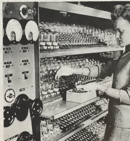
MACHINE SPRAYS MAGNESIUM OVER SMALL PIECES OF MICA USED FOR INSULATORS IN MINIATURE TUBES.
