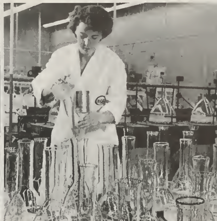
AN OPERATOR POURS FLUORESCENT SOLUTION INTO A GROUP OF 7-INCH CATHODE RAY TUBES.
