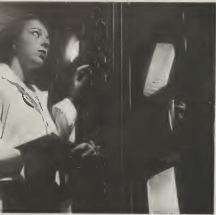
CHECKING KINESCOPE PICTURE TUBES DURING A 500-HOUR CONTINUOUS TEST.
