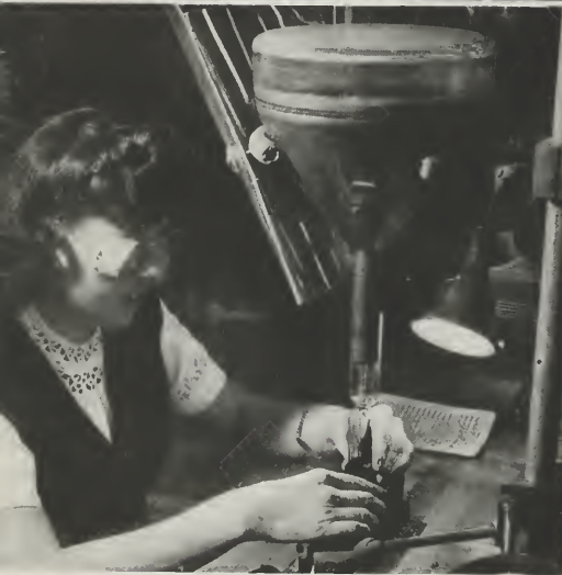
BELOW: NON-REFLECTING CARBON COATING IS APPLIED TO INTERIOR OF TUBE BY LONG-HANDLED BRUSH TO KEEP STRAY ELECTRONS FROM THE PICTURE SCREEN.
