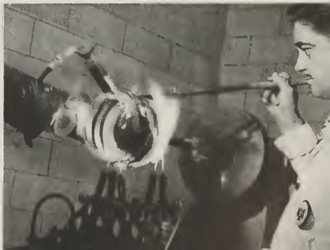
BELOW: USING THE INTENSE FLAME OF GAS BURNERS, THE GLASS FACE IS SEALED TO THE BACK OF A CAMERA TUBE.
