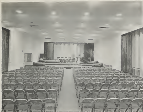
VIEWS OF NBC STUDIO 3A SHOWING UNEVEN WALL SURFACES WHICH CAN BE ADJUSTED TO CONTROL ECHOES.
