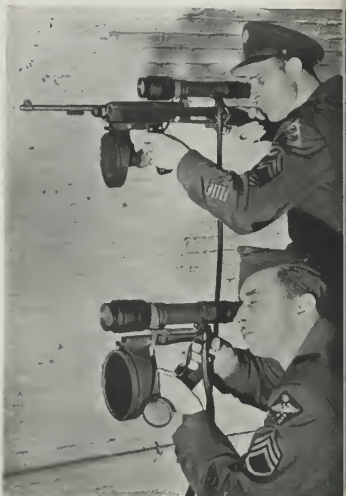
MEMBERS OF THE ARMED FORCES DEMONSTRATE THE SNIPERSCOPE (TOP) AND THE SNOOPERSCOPE.
