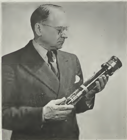
DR. V. K. ZWORYKIN HOLDS THE IMAGE ORTHICON WHOSE HIGH SENSITIVITY MADE POSSIBLE THE DEVELOPMENT OF AIRBORNE TELEVISION.
