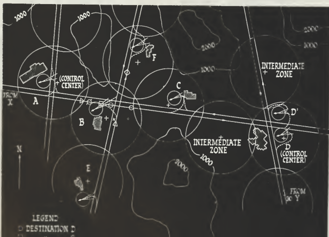
FIGURE 6—DRAWING OF COMPLETE TELERAN AIRPORT INSTALLATION COMBINED WITH SHORT-RANGE RADAR FOR CONTROLLING TRAFFIC. BELOW, FIGURE 7—PROPOSED NETWORK OF TELERAN STATIONS AS IT WOULD BE ARRANGED ALONG TRANSCONTINENTAL AIRWAYS, SHOWING OVERLAPPING RANGE OF EACH STATION.
