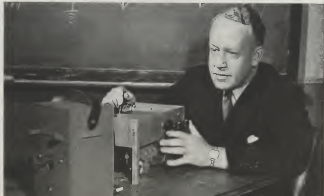
STUART W. SEELEY CONDUCTS TEST ON A RECEIVER CHASSIS EMBODYING A NEW FM RADIO CIRCUIT WHICH REDUCES THE NUMBER OF TUBES REQUIRED.
