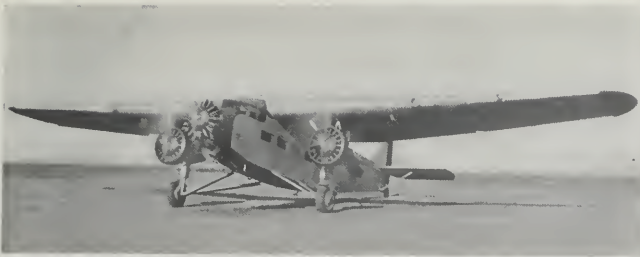
PLANE USED BY RCA FOR ITS OBSTACLE DETECTION TESTS IN 1937-39. THE V-ANTENNA APPEARS JUST ABOVE THE CENTER OF THE WING-SPAN.
