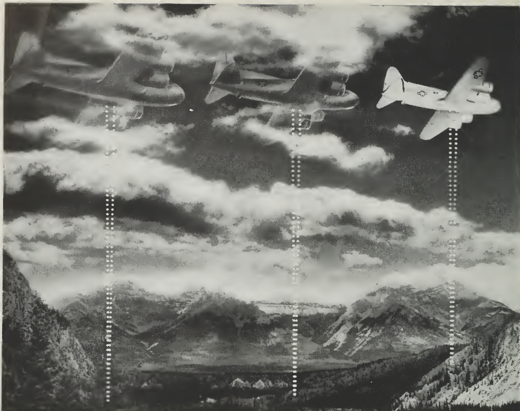
The RCA Radio Altimeter assures that the last mountains have been passed before letting down to the airport in the valley below.
