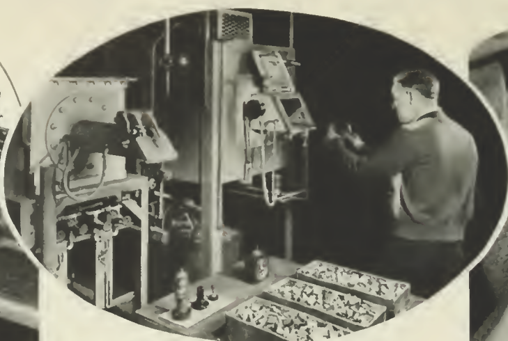
TURE PARTS ARE HEATED TO HIGH TEMPER- TURE IN THIS HYDROGEN OVEN.
