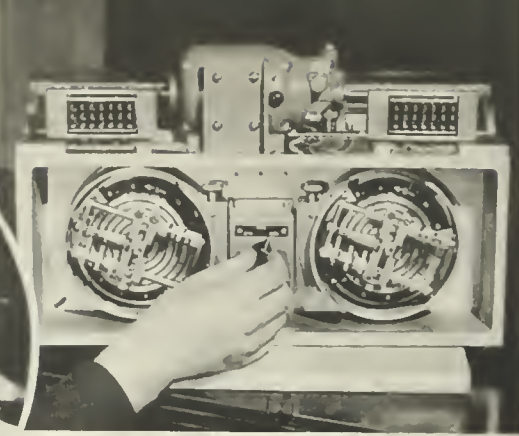
LEFT TO RIGHT: SEVEN-UNIT PRINTER AND PERFORATOR KEYBOARD USED WITH RCAC EIGHT-CHANNEL MULTIPLEX SYSTEM; MULTIPLEX DISTRIBUTOR WHICH ACCOMPLISHES MESSAGE SPEED OF 488 WORDS PER MINUTE; COW-BELL IN CENTER OF FRAME WARNS WHEN AN ERROR OCCURS IN TRANSMISSION.
