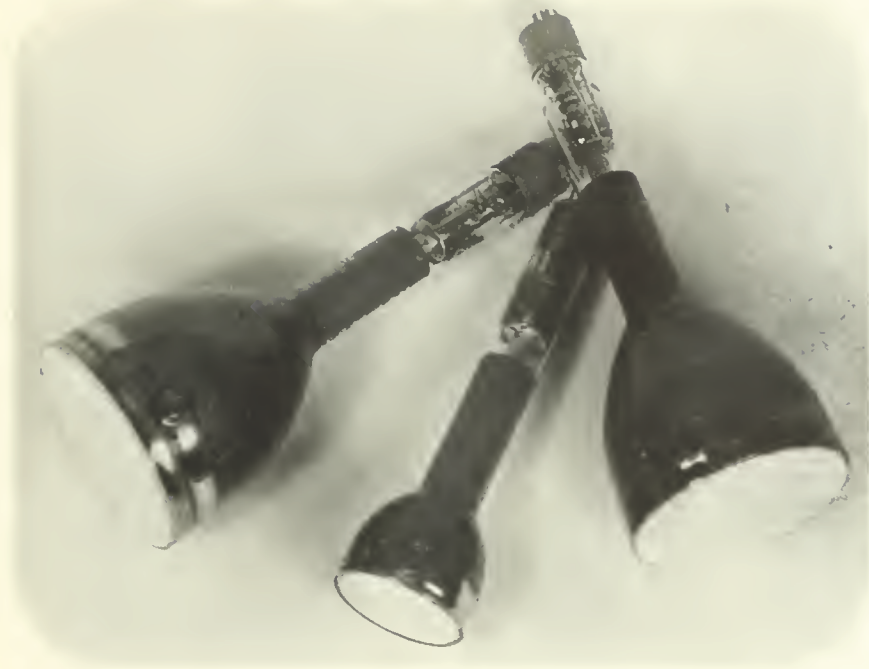
THREE LATE-MODEL KINESCOPIES FOR TELEVISION. LEFT TO RIGHT: 5-INCH FLAT-FACE AND 3-INCH FLAT-FACE FOR REFRACTIVE SYSTEMS; 5-INCH CURVED-FACE FOR REFLECTIVE OPTICAL SYSTEMS.
