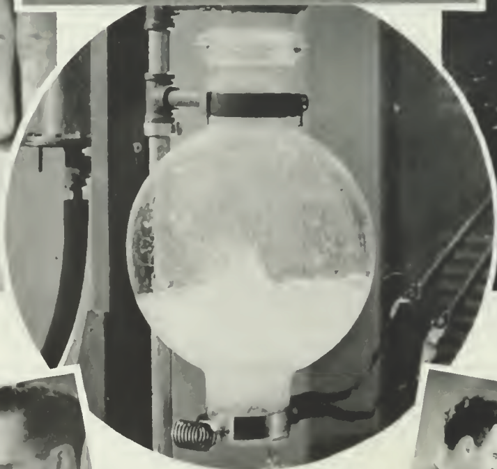
DEHYDRATING PENICILLIN BY MEANS OF RADIO-HEAT.
