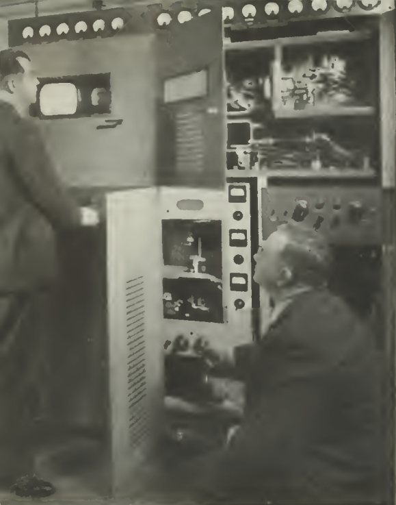
DEVELOPED IN RCA LABORATORIES, AN EXPERIMENTAL 300 MEGACYCLE TELEVISION TRANSMITTER IS PREPARED BY R. D. KELL AND T. L. GOTTIER, RESEARCH SCIENTISTS, FOR EARLY FIELD TESTS.
