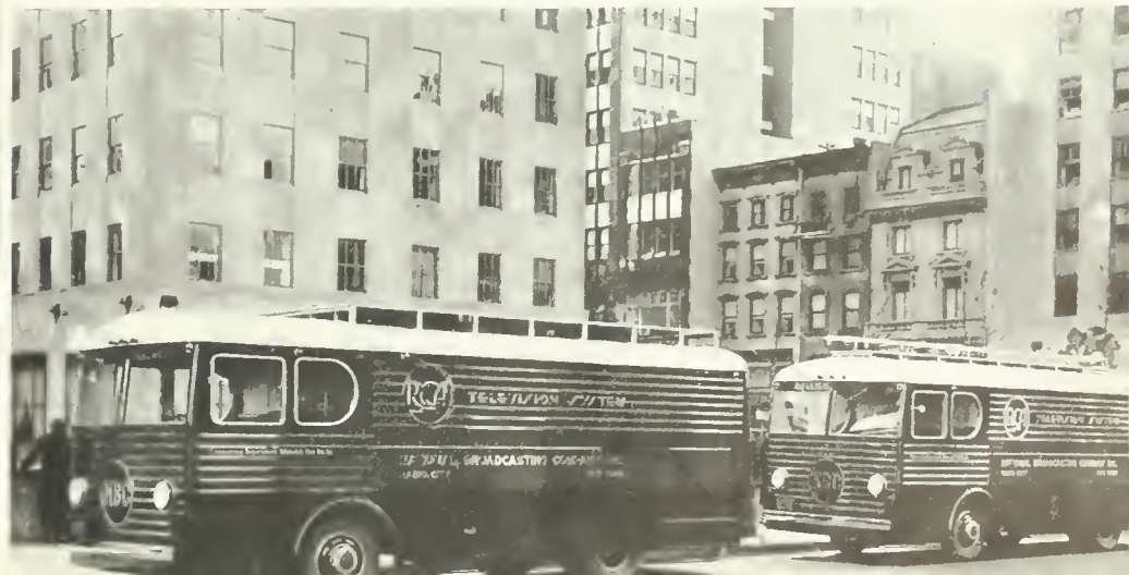
RCA PORTABLE TELEVISION EQUIPMENT (LEFT) IS SO LIGHT THAT A ONE-CAMERA UNIT CAN BE EASILY CARRIED IN AN ORDINARY PASSENGER AUTOMOBILE. BELOW—THE FIRST TELEVISION EQUIPMENT DESIGNED FOR OUTDOOR REMOTE PICK-UPS WAS INSTALLED IN TWO LARGE MOTOR VANS.
