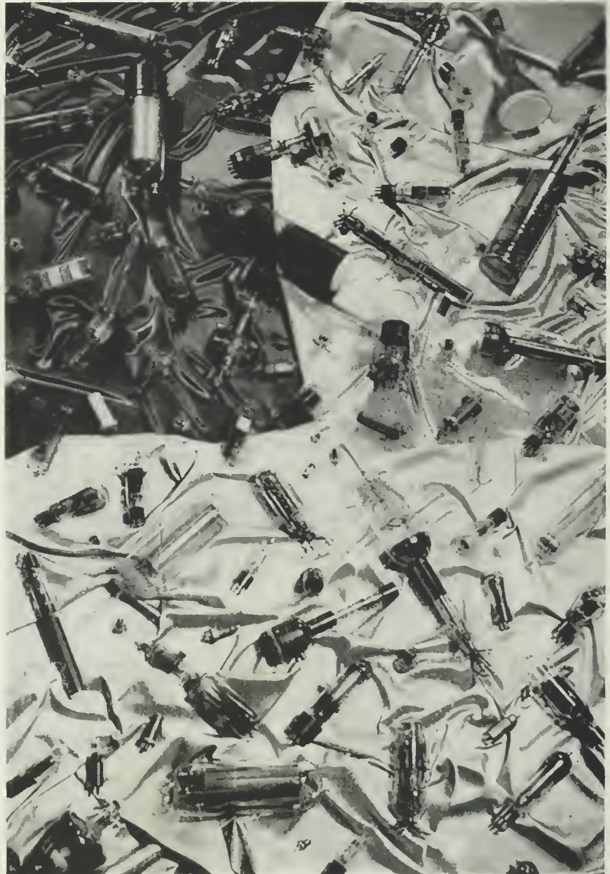
THIS DISPLAY OF TUBES REPRESENTS ONLY A FEW OF THE ULTRA-HIGH FREQUENCY POWER AND RECEIVING TUBES, CATHODE-RAY AND ELECTRON MULTIPLIER TUBES DESIGNED BY RCA RESEARCH MEN.
