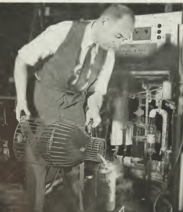
LIQUID AIR, TEMPERATURE 313 DEGREES BELOW ZERO, FAHRENHEIT, IS USED BY J. BURNETT TO IMPROVE THE VACUUM IN A TUBE WHEN IT IS COMPLETED. BELOW, H. A. FINKE TAKES PERFORMANCE DATA ON A RESEARCH TUBE AS IT IS PUT THROUGH ITS PACES IN AN ELABORATE SERIES OF ELECTRICAL TESTS.
