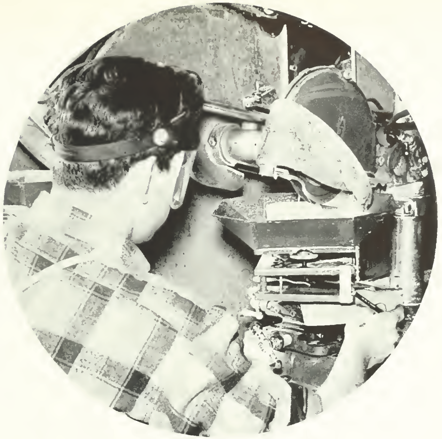
DIAMOND SAW OPERATOR AT CAMDEN PLANT OF RCA VICTOR DIVISION, CUTTING A NATURAL CRYSTAL WHICH, AFTER PROCESSING, WILL CONTROL RADIO AND ELECTRONIC APPARATUS.
