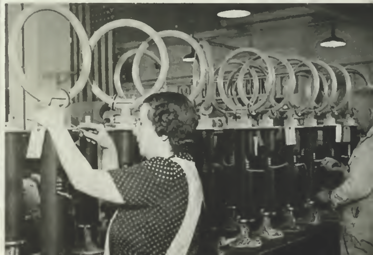
THESE SMALL RADIO DIRECTION FINDER LOOPS ARE BEING COMPLETED BY RADIOMARINE FOR WAR SERVICE AT SEA.
