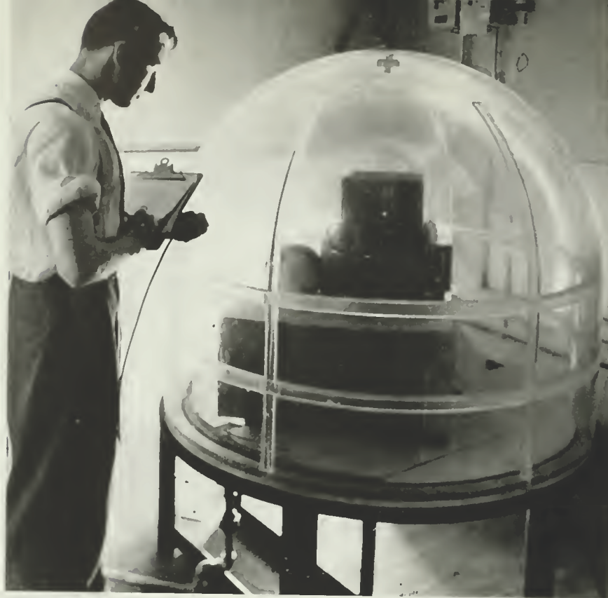
TECHNICIAN RECORDS OPERATING DATA FROM THE COMMUNICATIONS UNIT BEING TESTED IN THIS RECENTLY DEVELOPED ALTITUDE CHAMBER.
