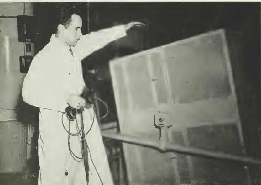
COMMUNICATION EQUIPMENT IS SUBJECTED TO THE POUNDING OF A SLEDGE HAMMER (ABOVE), SIMULATING GUN RECOIL. IN THE "TUMBLER" TEST (BELOW), A ROTATING BOX IN WHICH RADIO AND SOUND UNITS MAY BE DROPPED 1,000 TIMES, IS USED.
