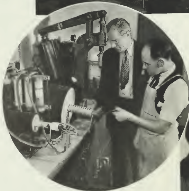
FROM THIS HIGH-TEMPERATURE FURNACE USED IN METALLURGICAL INVESTIGATIONS OF RADIO CIRCUIT COMPONENTS, C. WENTWORTH AND W. L. CARLSON PREPARE TO REMOVE A TEST SAMPLE.
