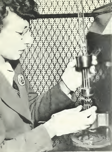
INSTALLING THE GRID STRUCTURE OVER THE FILAMENT (LEFT) IS A PART OF THE TUBE REBUILDING PROCESS; THEN COMES THE PREPARATION OF THE COPPER ANODE TO WHICH THE GLASS BULB IS TO BE SEALED (CENTER), AND THE ACTUAL SEALING (RIGHT) OF BULB AND ANODE.
