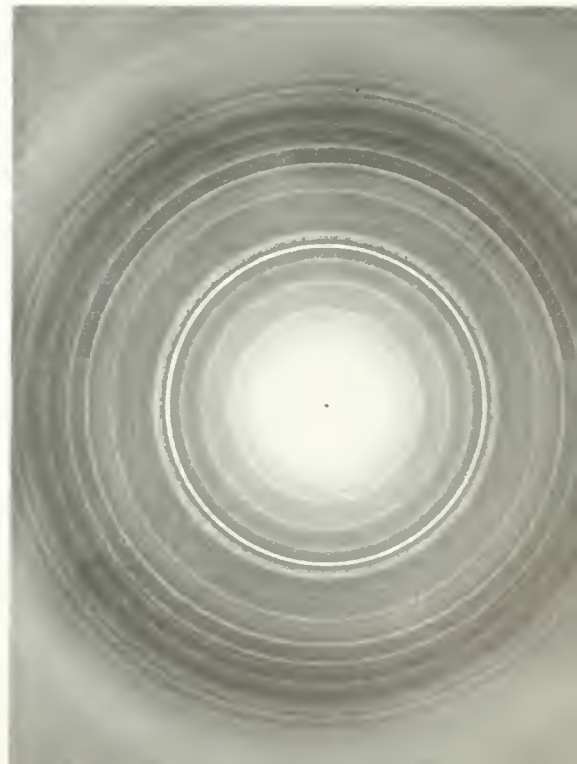
DIFFRACTION PATTERN OF ZINC OXIDE OBTAINED WITH THE ELECTRON DIFFRACTION CAMERA ATTACHMENT OF THE MICROSCOPE.
