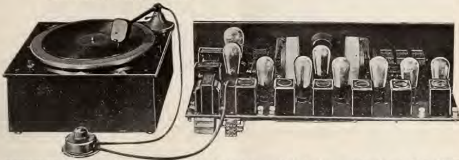
Method of attaching the World's Record Super 10 receiver to the phonograph to get richer, sweeter music out of the whirling record
