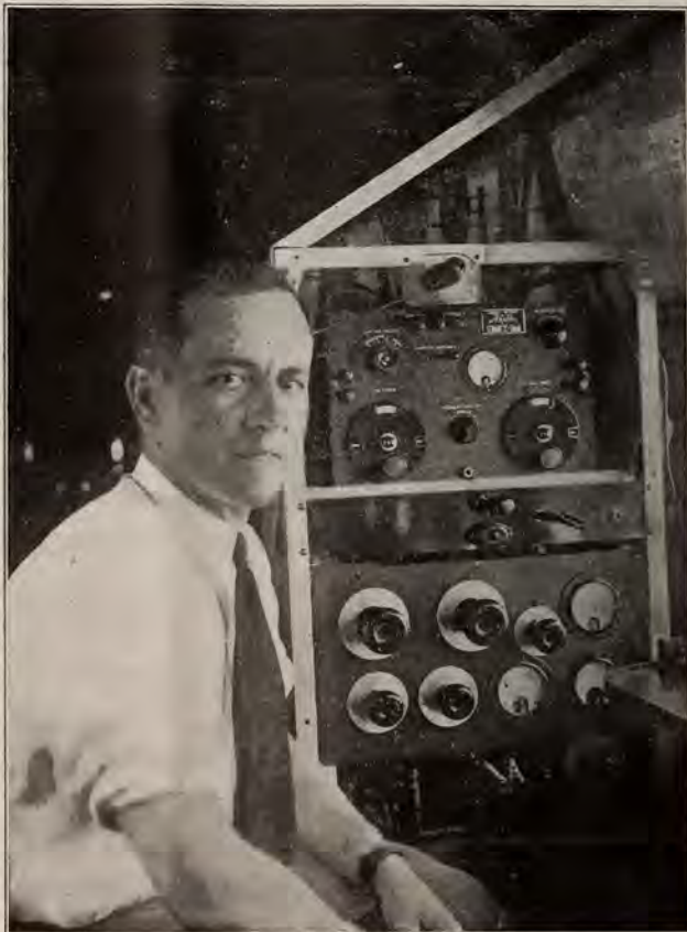
Ensign S. V. Edwards, U. S. N., seen at the radio set he will operate in the huge Sikorsky plane recently built for trans-Atlantic flights. The set is designed to be capable of sending and receiving messages from France or the United States as soon as it takes the air, having both a low and long wave length. The set weighs 125 pounds and was built by the Washington Navy Yard.—Photo copyright by Henry Miller.
