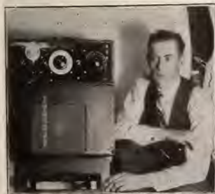
After it is thoroughly tested, it can be mounted on good panels and placed in a neat portable case with built-in loop and loud speaker
