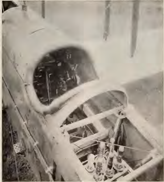
Radio installation in aircraft, mail-carrying transport, showing transmitter, reel and control box
