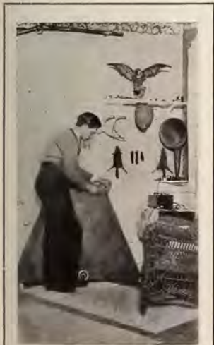
Roy Bates of Plattsburg, New York, uses a copper tank from a wrecked rum runner for an indoor aerial.
