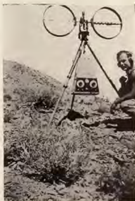
The "radiore" set in operation in the field. Notice the direction-finding loops
