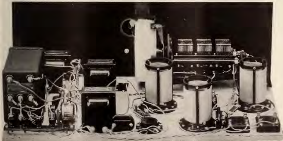
Rear View of A. C. Operated Receiver Showing Placement of Parts and Associated Wiring. The Set is Wired with Flexible Rubber Covered Wire, Simplifying Wiring and Construction. The 171 Bias Resistor and By-pass Condenser are Hidden from View Behind the Out-put Transformer.
