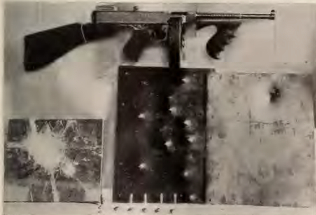
Interesting exhibits showing effect of gun bullets on Bovite sheets. Above is shown the Thompson machine gun used in all tests. Lower left, bullet proof glass which stopped 6 bullets in one spot. Center, sheet of Bovite (less than 1-16 inch thick) which stopped every bullet. Right, another 1-16 inch sheet of Bovite showing reverse side and two bullet marks. Bottom, cartridges and used steel bullets, showing how they are deformed. Two at left, all that could be found of the 6 bullets fired into the glass. Five others were fired against the sheet of Bovite. Ranged at the rear, for comparison, are unused cartridges
