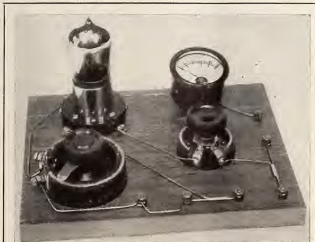
Photograph of the completed vacuum tube voltmeter described by the author
