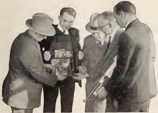
Jim Letts, the "human target" who has been shot 5,000 times and never wounded. He has ripped away the cloth covering and is showing the marks of 17 machine gun bullets just fired at his body. Some of the bullets may be seen still adhering to the bullet proof vest. One man holds some of the deformed bullets in his hand
