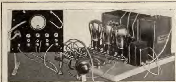
In this picture is shown the testboard (left) and the full wave 216-B combination which gives power for both the broadcast receiver and the low power crystal transmitter. The meter in the test board is a milliammeter which may be plugged into any of the voltages supplied either the broadcast receiver or the transmitter
