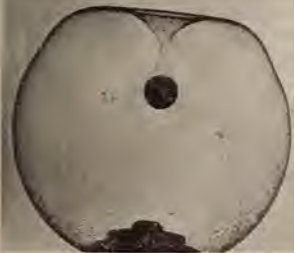
STEEL BALL DROPPED IN A SOAP BUBBLE. This photograph, made about a hundredth of a second after the ball first touched the bubble, shows that it has not yet begun to break, but extends down around the ball like an elastic membrane
