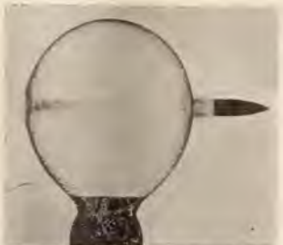
THE BULLET AND THE BUBBLE photogr aph made in the sound laboratory of the U. S. Bureau of Standards by means of an electric spark, by Philip P. Quayle, showing a soap bubble through which has been fired a rifle bullet. The bullet has passed out of the bubble, but it still stands, with a hole in each side. The lines extending from the front of the bullet are sound waves
