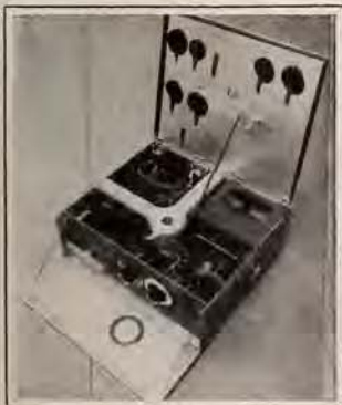
Photograph showing the completed portable direction finder developed by Mr. Dunmore, having a wavelength range from 39 to 3,300 meters
