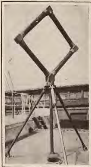
View of radio compass loop mounted on upper deck of vessel. Rotation of the loop is controlled from inside the cabin beneath.
