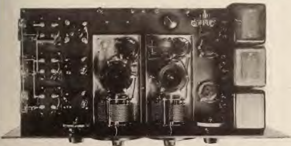
Photograph of the completed Clough superheterodyne with the stage shields removed from the first detector and oscillator
