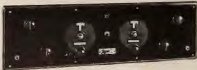
Front panel view of the Microflex, showing the switch located at center of panel
