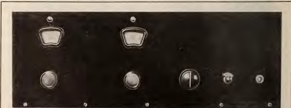
This front view of the receiver shows the Marco controls, Centralab variable resistor across the first audio grid circuit for volume control, then the Yaxley switch and the phone or loudspeaker jack. The little knobs above the Marco controls are for turning on and off the lights back of the celluloid dials, current being taken from the same source as for the filaments
