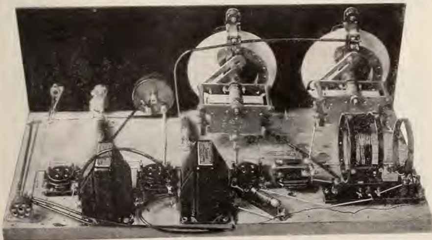
Rear view of the completed short-long wave receiver showing Marco illuminated controls, Aero plug-in coils as well as other units mentioned in the text of the accompanying article
