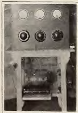
Front panel view showing meters and dials, while helix is shown on lower shelf
