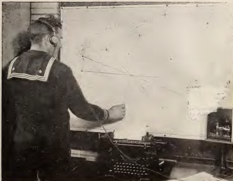
Operator at control station plotting bearings on ship taken by several compass stations. Where the strings converge is the location of the vessel
