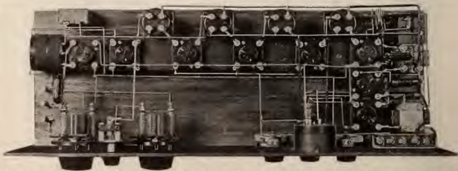
Top view of the Radio Age laboratory model World's Record Super 8 showing all parts wired in place in accordance with the schematic circuit shown on page 40
